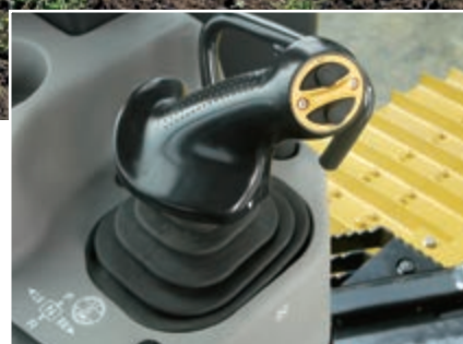
Commandes ergonomiques PCCS (Palm Command Control System)
